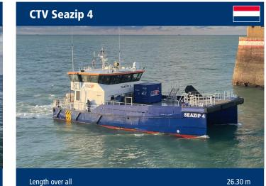
Length over all Passengers Yard / Year built Damen Shipyards / 2015 2 x Caterpillar 895 kW Engine Service speed
