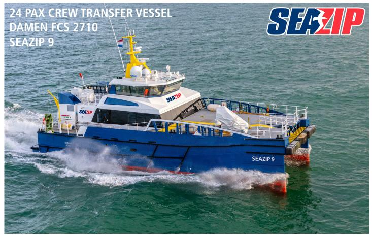
MV SeaZip 9 is a fast Twin Axe Bow catamaran for transport of Industrial Personnel, equipment and parts to offshore windfarms and oil & gas fields.
