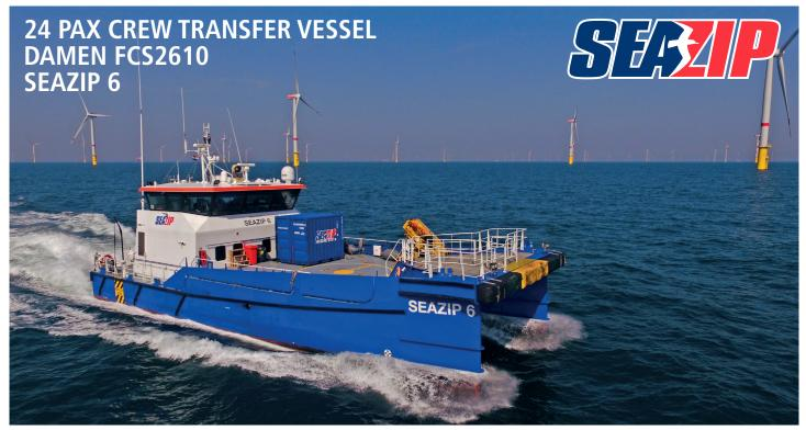
MV SeaZip 6 is a fast Twin Axe Bow catamaran for transport of Industrial Personnel, equipment and parts to offshore windfarms etc.
