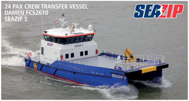
MV SeaZip 5 is a fast Twin Axe Bow catamaran for transport of Industrial Personnel, equipment and parts to offshore windfarms etc.
