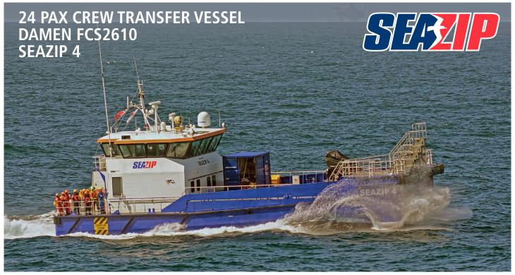
MV SeaZip 4 is a fast Twin Axe Bow catamaran for transport of Industrial Personnel, equipment and parts to offshore windfarms etc.
