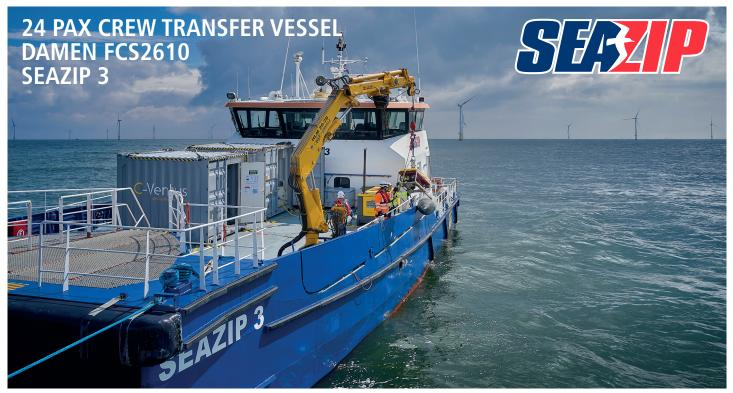
MV SeaZip 3 is a fast Twin Axe Bow catamaran for transport of Industrial Personnel, equipment and parts to offshore windfarm etc.
